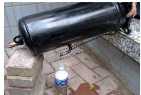
Step 2: Inspect oil from faulty compressor
