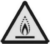
The A2L logo on the nameplate indicates that the product contains refrigerant of the slightly flammable category. It is also positioned on schraders where refrigeration components can be connected for maintenance. This label tells you that there is a potential risk of a flammable gas leak and that this should be taken into account in the operational risk analysis.
