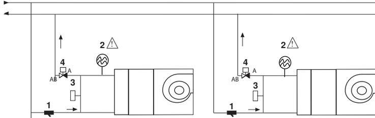
UNITS INSTALLATION WITH THREE WAY VALVES. (UNITS 007 to 040 and 002-003 LWT version).
