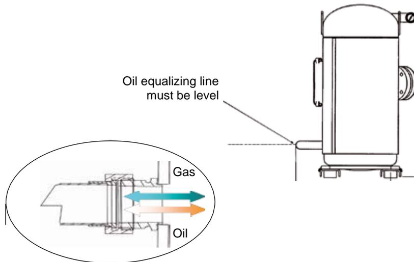
The oil equalizing Line is fitted with a sight glass which can be used to check the oil level in the compressor assembly. It is mandatory to stop both compressors to get a good reading of the oil level in the crankcase of the compressors.
