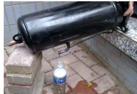
**Step 2: Inspect oil from faulty compressor**
