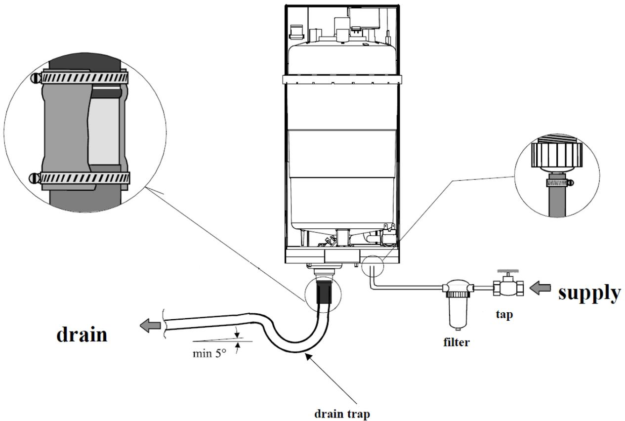
To simplify installation, it is recommended to use hose with an inside diameter of 6 mm and an outside diameter of 8 mm and the revolving 3/4" G connection, either straight or 90°.
